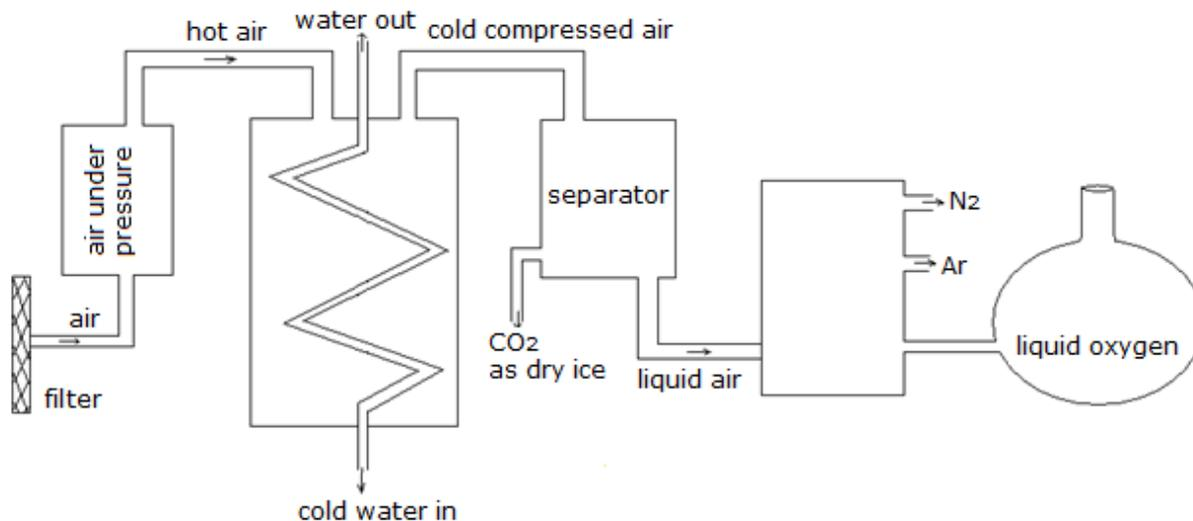
separation of components of air
